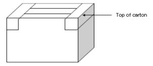
Carton sides should be secured using an adhesive type sealant (i.e. glue, tape, etc) vs. stapling as this is more durable and minimizes risk of damage to associates and merchandise. If cartons experience a high rate of bursting during transit (>3 occurrences), the Company may mandate a specific carton closure method.
